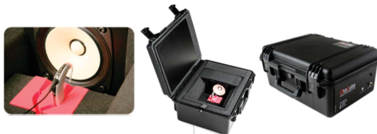
Figure 1. Portable desktop box (Otocube) used in audiometric examinations of cochlear implant users.
